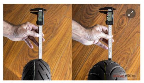
In our measurements, the front and rear Protorq tyres weighed around 4kg and 5kg, respectively. And in terms of tread depth; these measured over 4mm and 5mm, front and rear. Additionally, the Protorq Extremes are W rated tyres. And they use a dual compound construction to offer both good centre tread life, and fantastic edge grip.
