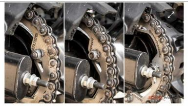
Says Joshua, "Step one was to centre the rear alloy for it to sit correctly in between the swingarm. This meant fabricating bespoke spacers. Then came a new sprocket to fit the new wheel. The number of teeth remains identical to the stock sprocket, of course, but the new customised unit is lighter and less prone to wear.'
